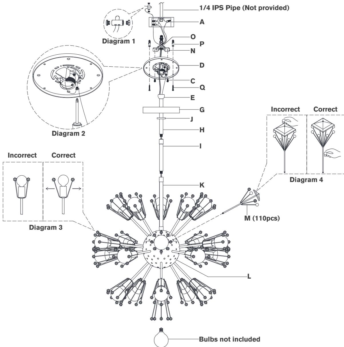
20. Install canopy (**G**) to mounting plate (**D**) and secure with collar ring (**J**).
